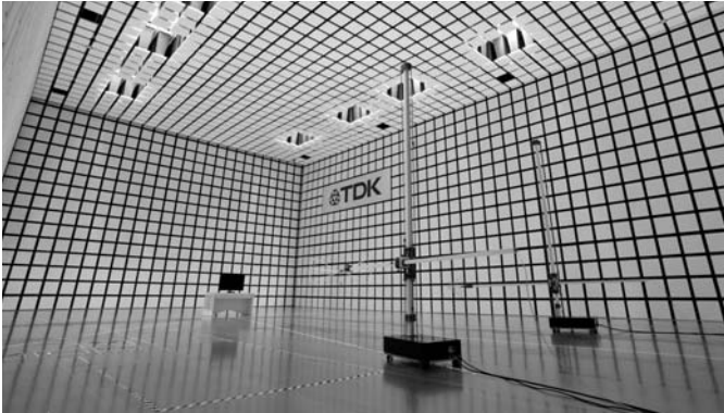
10-meter test range anechoic chamber (uses IP material for radio wave absorption)
